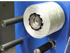
Our pneumatic bobbin adaptors can be mounted on already existing 3-inch bobbin shafts of almost every creel system. The outside is made of an expandable rubber with aluminum strips which expands by using of compressed air.
